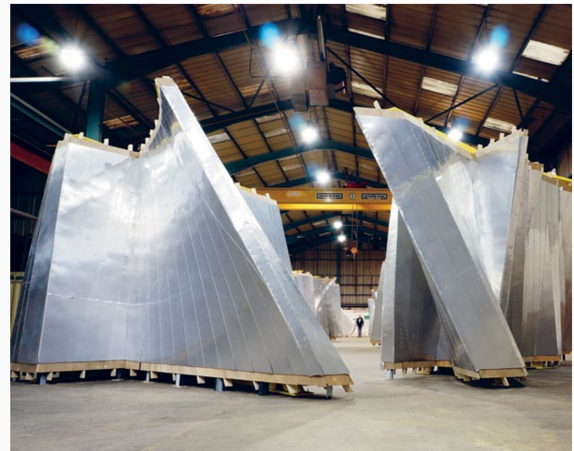
Above: Three connecting cassettes being put together for the first time for a factory presentation in Hull. Left: Slipstream production at Hull factory prior to delivery to Heathrow
