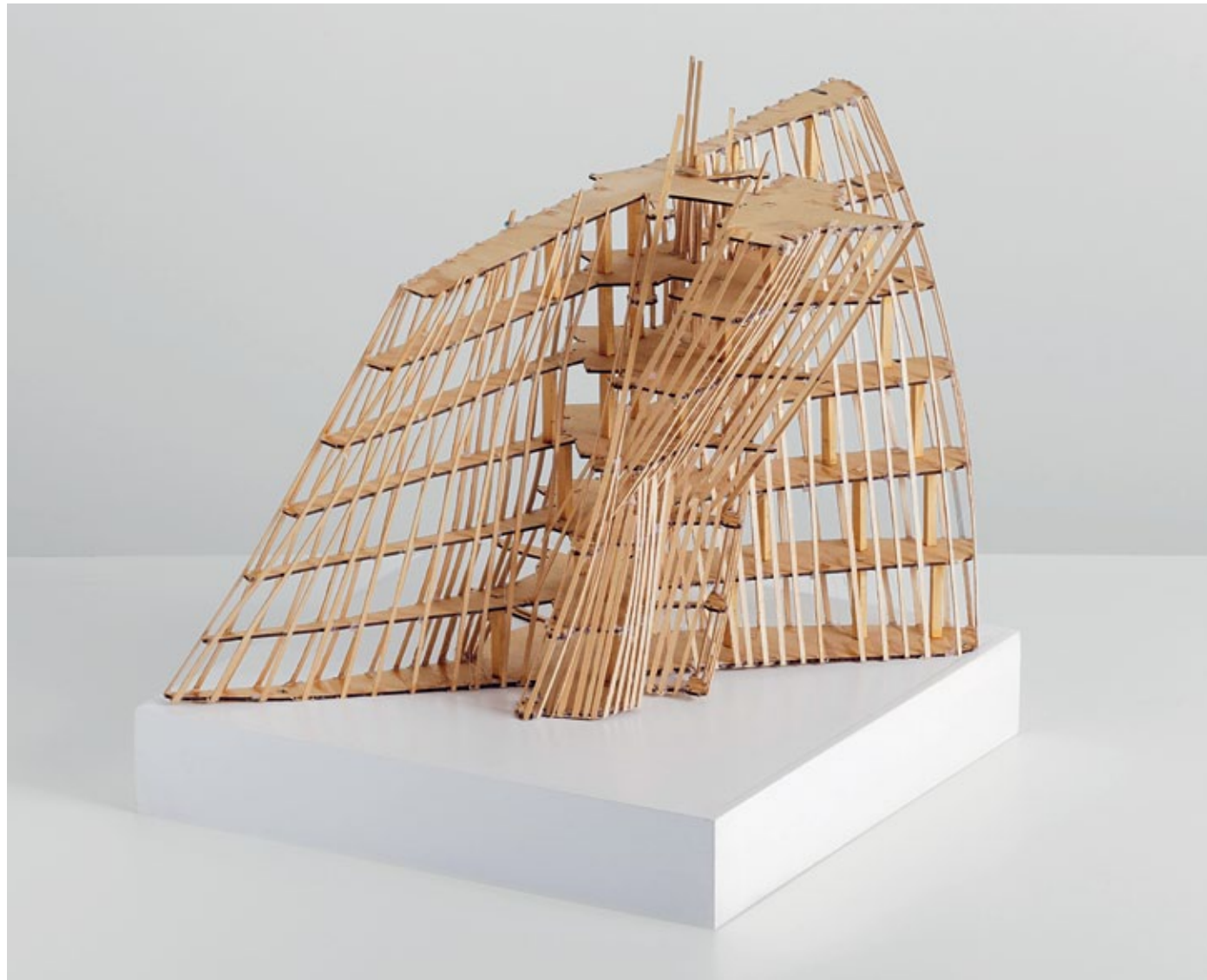
Above: Unfinished scale model of cassette incorporating bulkhead and combs, pictured in an upright position (not the correct horizontal position). Right: Price & Myers drawings detailing laminate and fastening of the aluminium skin. Opposite page: Sequential development of a single cassette from steel armature to aluminium skin
